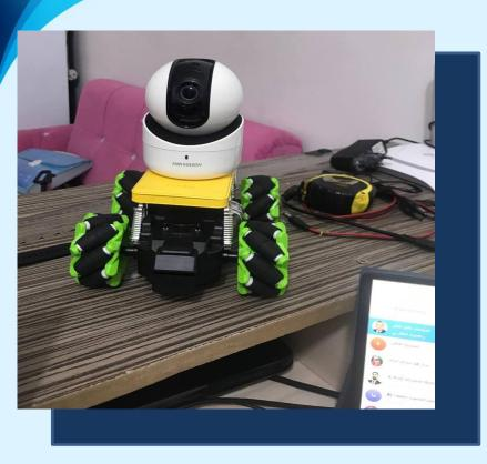
A simple robot to assist the visually impaired in navigating inside the home to avoid obstacles, guiding the visually impaired to their destination within the home, as well as identifying the types of entities around them. It can identify more than 40 entities or materials inside the home (such as kitchen tools, people, furniture, and others).
