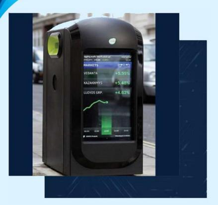
A smart waste container, advanced practical device for automatically throwing and separating waste, placing it in the appropriate place for easy recycling. It notifies when the waste level is full and is equipped with a voice feature to thank the user and alert about the type of waste.
